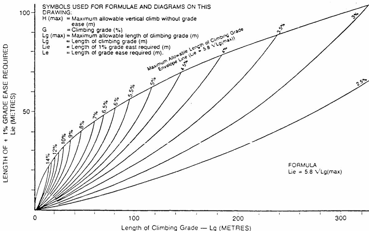
Note: Figure 10a shows the minimum length of +1% grade ease,  $L_{ie}$ , required for each particular length of climbing grade,  $L_g$ , at various different climbing grades,  $G$ . Where the climbing grade is not constant, a series of lengths,  $L_i$ , of different climbing grades,  $G_i$ , may be used provided that:
